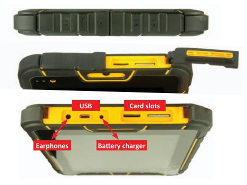
The tablet can be charged by inserting the battery charger cable into the charger port on the top, and connecting the plug to the mains power supply.
