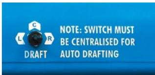
This switch manually opens and closes either the left hand or right hand draft gates.
