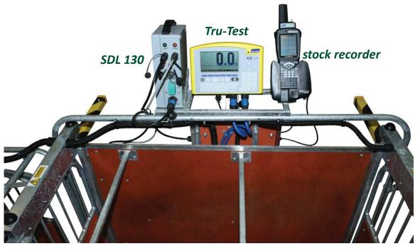
Set the SDL 130, the Tru-Test weigh scale and the stock recorder into their mounting brackets.
