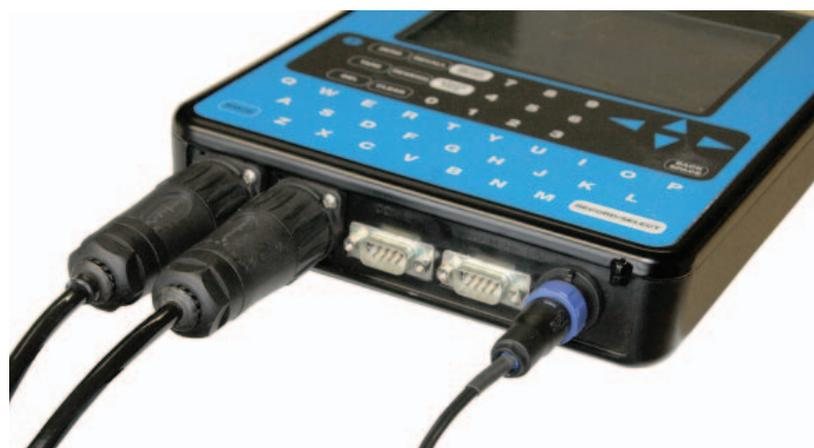
*Two heavy black cables from the load bars under the crate connect to the weigh scale. The third cord is lighter, with a threaded blue collar that fits into a smaller socket. Tighten all connections.*
